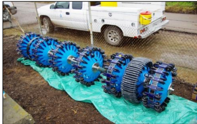
Figure 5 - RAFT in-line inspection tool used for the 36-inch Aqua Connector.
