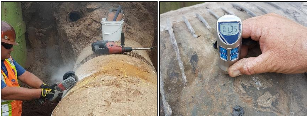
Figure A1. The mortar liner was removed by AWD technicians at the reported site of the corrosion (left). A UT probe was then used to measure the depth of the observed external corrosion in Segment 149 (right).
