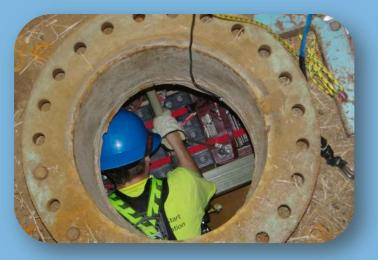
The tool is completely self-contained with battery power, data storage and distance tracking all integrated on the tool itself. Target pipe applications are internally lined (cement, coal tar, epoxy) steel pipe, riveted pipe, lock-bar pipe, Cement Mortar Lined and Coated (CML&C) Steel Pipes and Bar-Wrapped Steel Cylinder Concrete Pressure (AWWA C303) Pipes.
