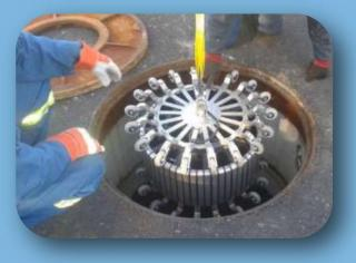
Depending on tool size and access availability, the tools can be directly loaded into the pipeline through a manhole or an open pit, or they can be inserted through a manhole in smaller modules and assembled inside the manhole chamber. The Chimera tools can be tethered on both ends and winched through pipeline sections up to 6,000 feet. Where conditions allow, the smaller tools (16-inch to 24-inch) can be deployed in a free-swimming mode and travel longer distances between access points.
