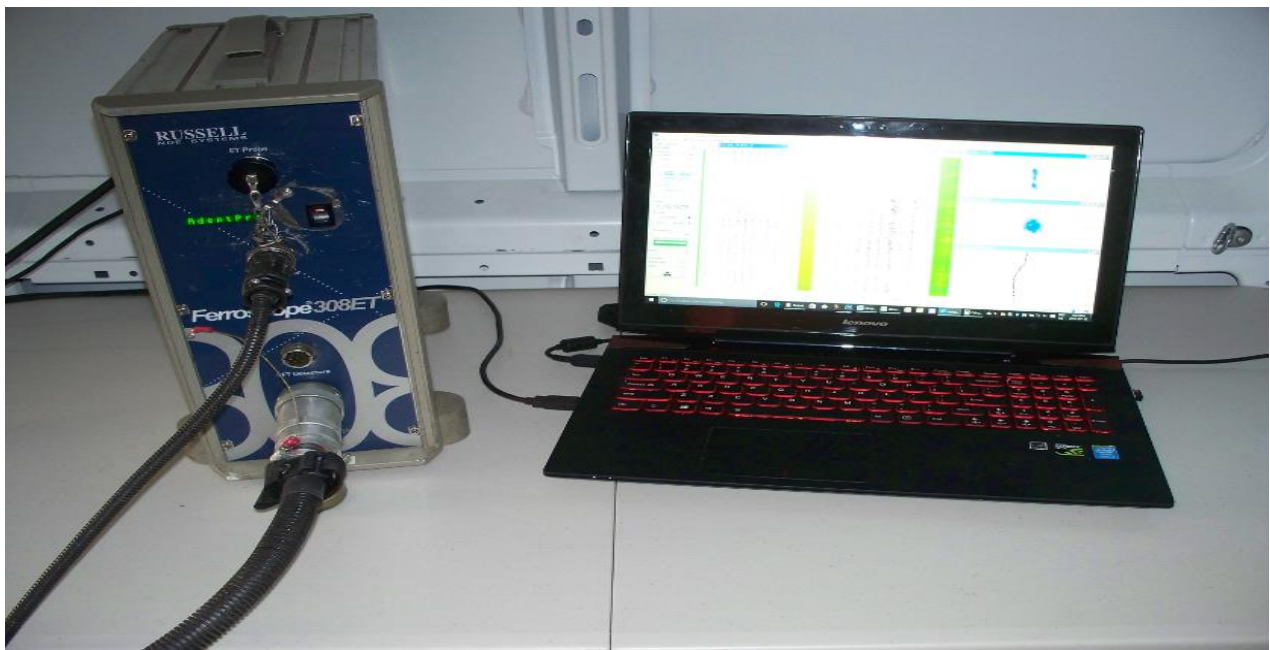
Figure A2-4. Typical setup for Ferroscope and Laptop computer at job site.
