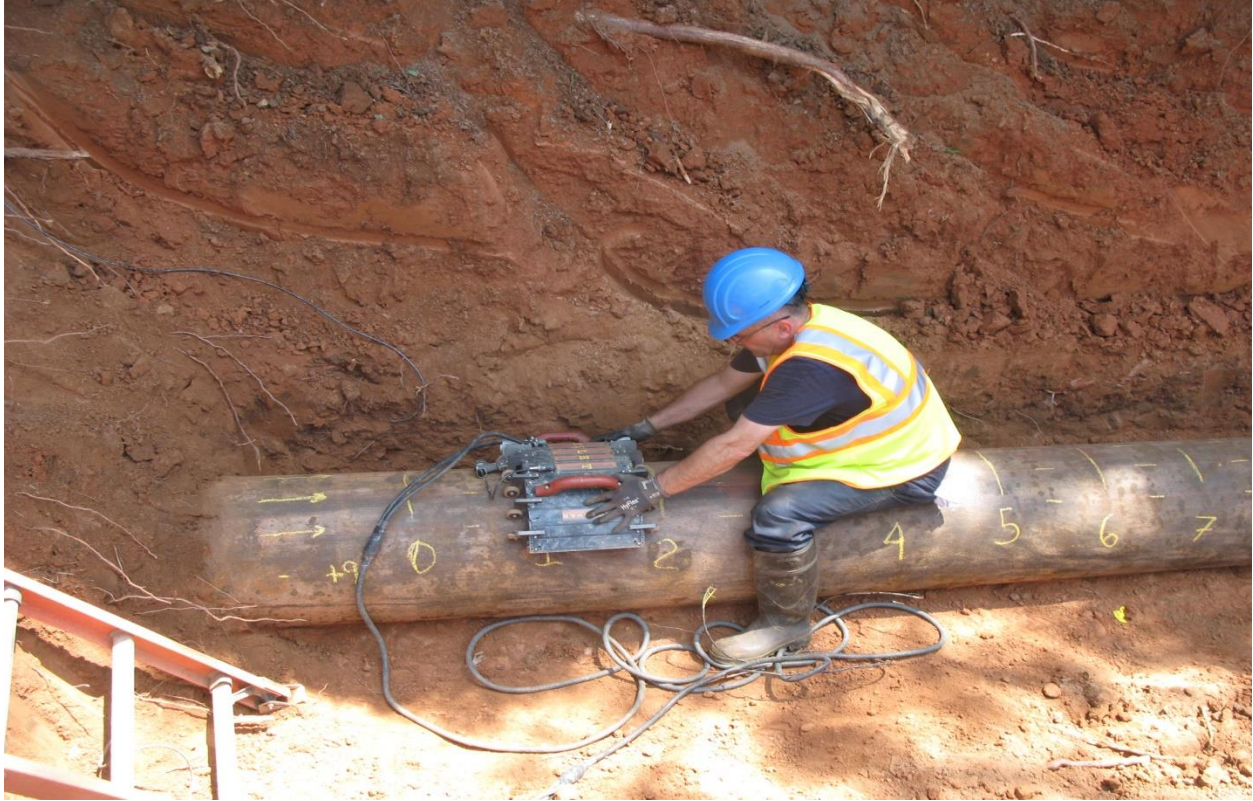
Figure A4 Typical BP scanning technique.
