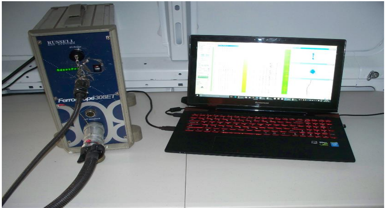
Figure A2-4 Typical setup for Ferroscope and laptop computer at job site.
