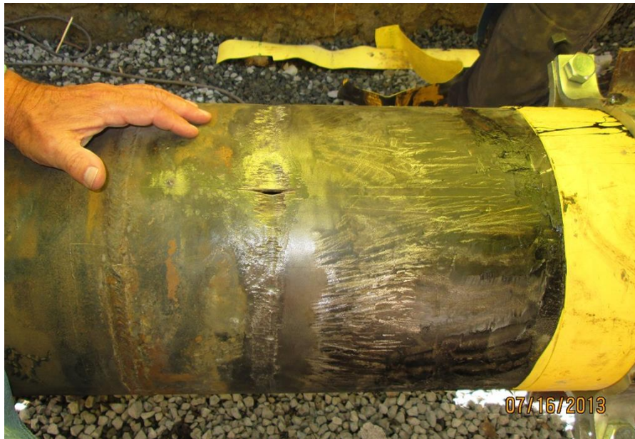
Figure 6: Examining AOI 3b showing a through hole at the 9 o'clock position
