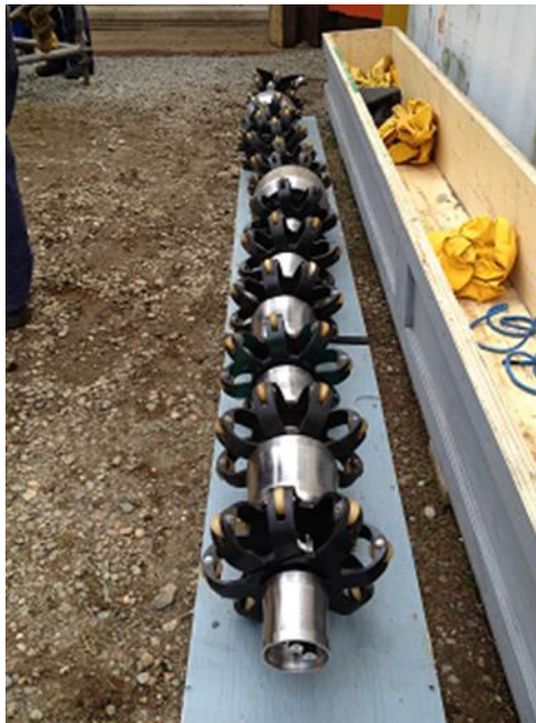
Figure 2: Picture of the See-Snake inspection tool
