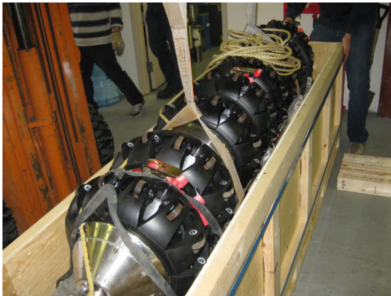
Fig-5: Typical RFT Tool (courtesy PICA Corp)
