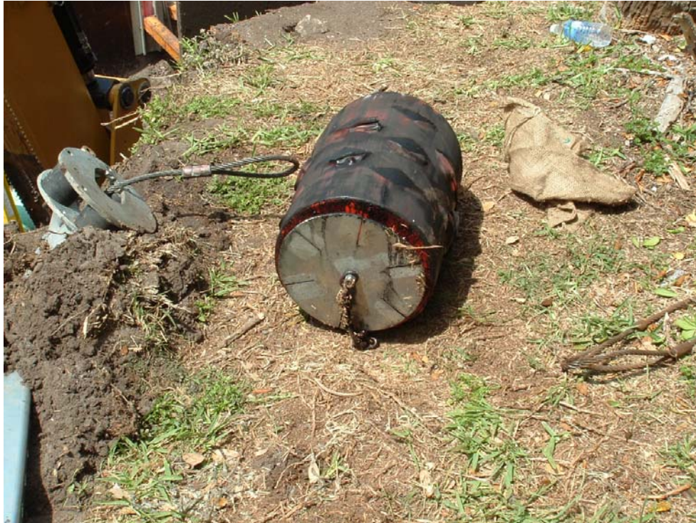
Fig-5: shows no damage on the sizing plates (that are slightly larger than the actual inspection Tool)
