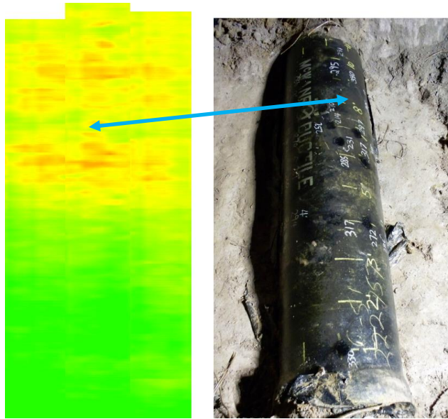
Figure 2. Inspection results for a segment FM pipe
