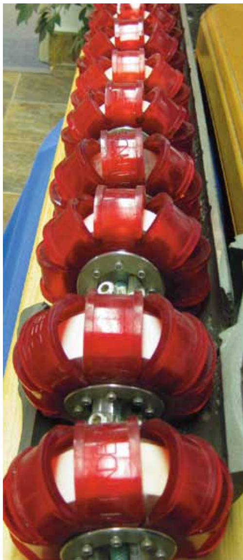
Figure 2. A typical RFT ILI tool.
