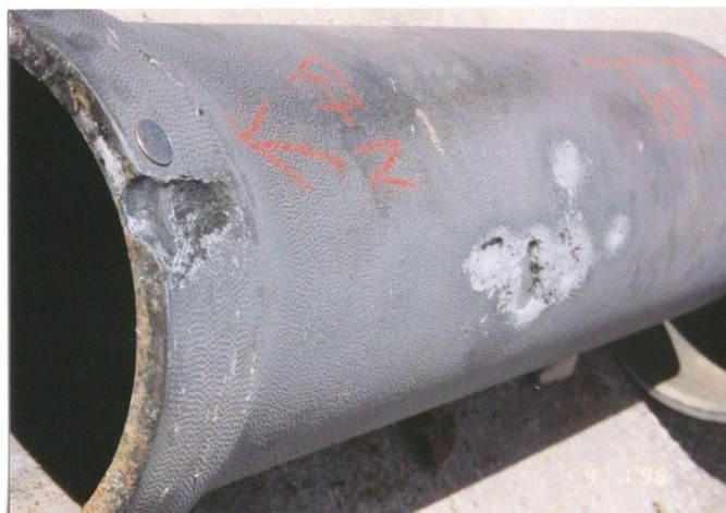
Fig-1: typical corrosion cells in cast-iron pipe
