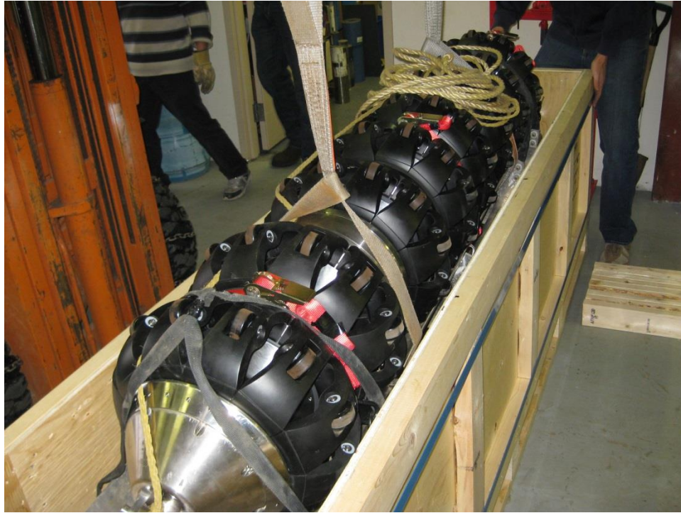
Fig-3: Typical 16" pipe diameter RFT Tool (courtesy PICA Corp)
