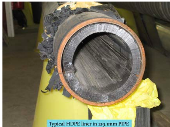
Figure 3: Lined Sour Gas Pipelines - ILI Technology Challenge
