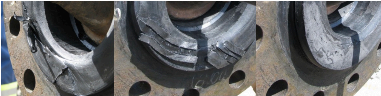
Figure 9: Left to Right; Damaged liner flange stub end, HDPE filler strips applied to fill areas of material loss and Finished stub end after sanding
