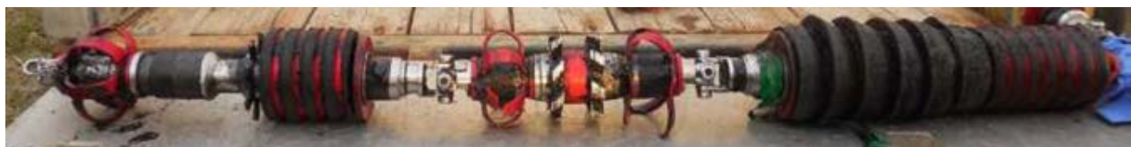
Figure 10: Custom Tow Pig/Reamer/Gauge Pig used in the CML Pipeline
