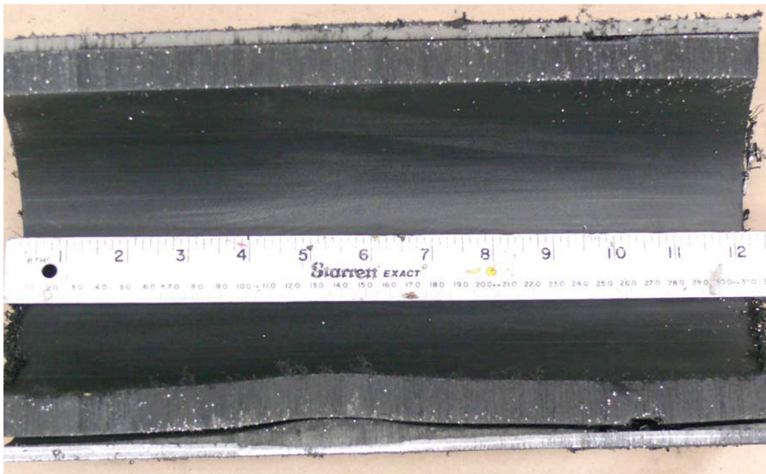
FIGURE 4 - Scale build-up and Metal loss at Bulge in Pipe Cut Out
