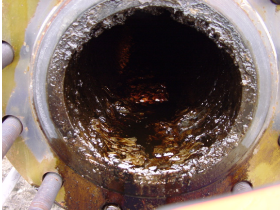
Fig-5a) and 5b) Wax, Sand and Oil deposits in O&G line
