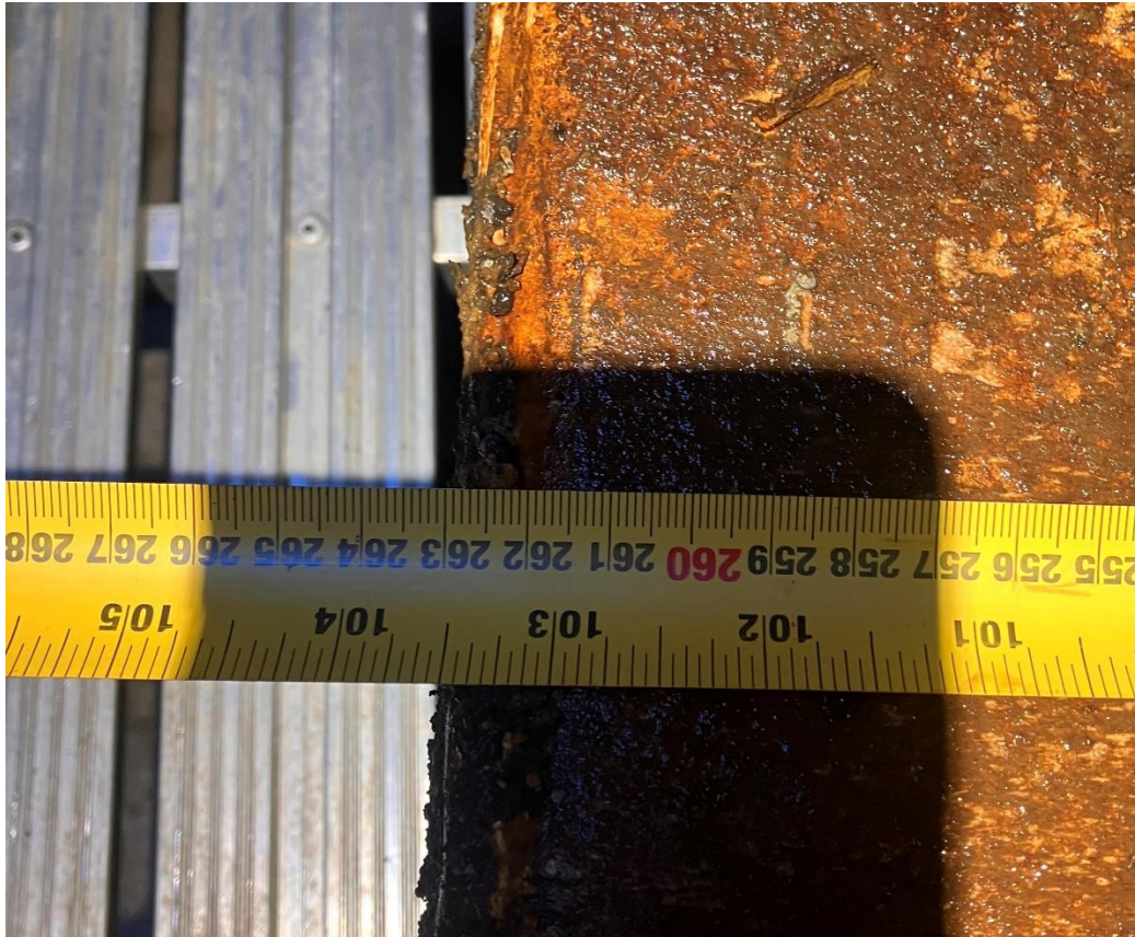
Figure 10 – Confirmation of the joint gap spacing begins at 103.5-inches (2.62m)
