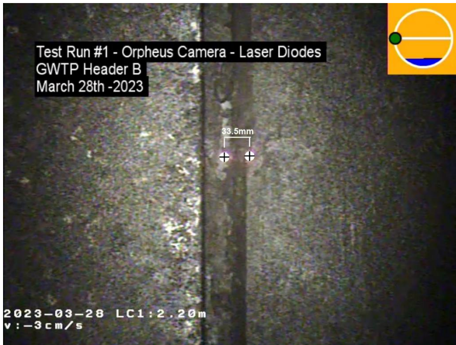
Figure 13 – Laser Diode Measurement of Gap at the 9:00 position -50 mm
