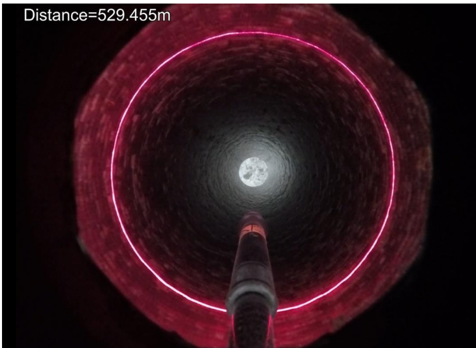
Bottom Image: The hard-facing liner is easily seen before exiting at the bottom at the mine
