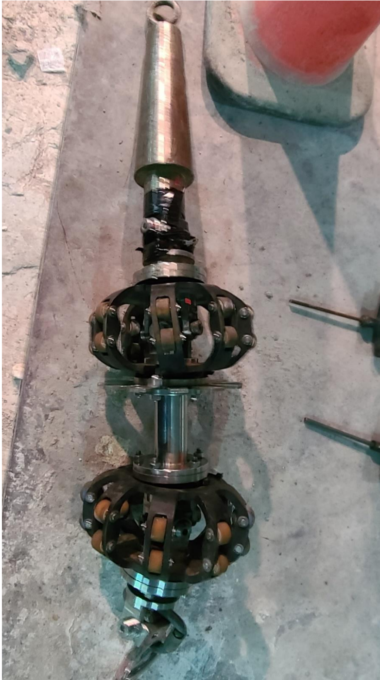
Figure 5. Gauge tool assembly used on Slick Lines #1 and #2 prior to the main inspection
