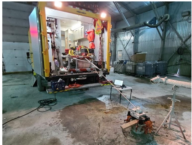
Figure 2. Typical setup on Slick Line using a winch and rollers to guide inspection tool down the pipe
