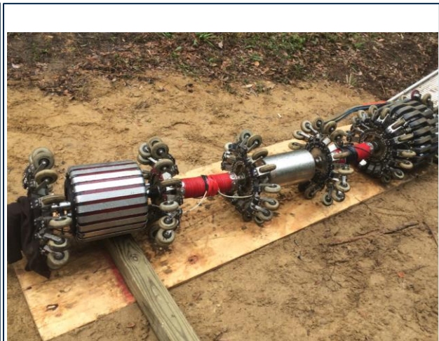
Figure 2b: PICA's Chimera tool used for larger diameter inspections.
